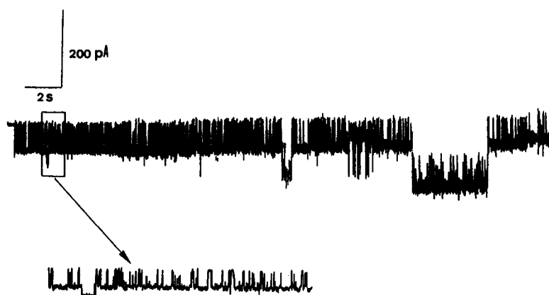
Fig. 5. Trace of current fluctuations of OmpA2 protein ( 10^{-9} M) in 0.25 M KCl. Applied voltage V = 50 mV. Digitization rate: 5000 Hz and filter: 100 Hz.
